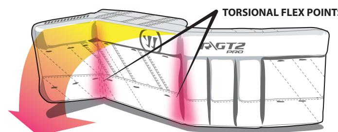
TORSIONAL FLEX POINTS BELOW THE KNEE AND ANKLE ALLOW THE TAPERED BOOT TO TILT FORWARD AND SEAL ALONG THE ICE WITHOUT CAUSING THE THIGH RISE TO LIFT
